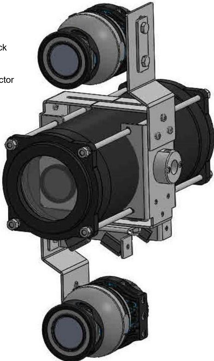
Shown--Sony HD block camera and SeaLite Sphere lights
